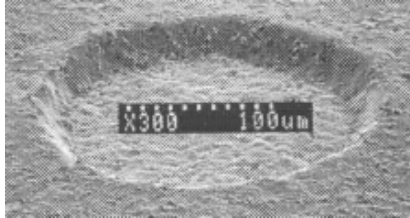
Fig. 6.12 300 x SEM micrograph of developed via formed in fired Q42DP after Reference 14. (Courtesy of Du Pont)
